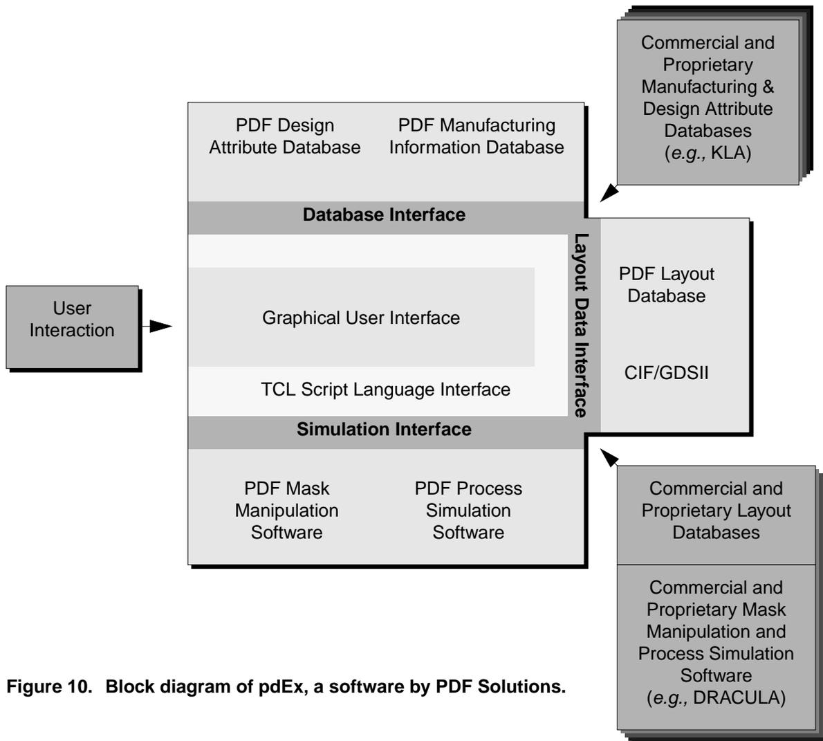
Figure 10. Block diagram of pdEx, a software by PDF Solutions.
