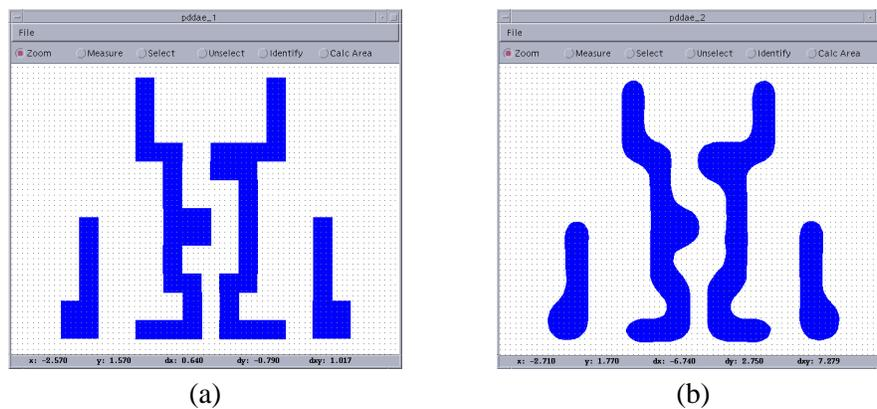
**Figure 2.** Models of the polysilicon gate layer for an SRAM cell. (a) shows the drawn mask layer, (b) shows the printed imaged as modeled by aerial imaging simulation.
