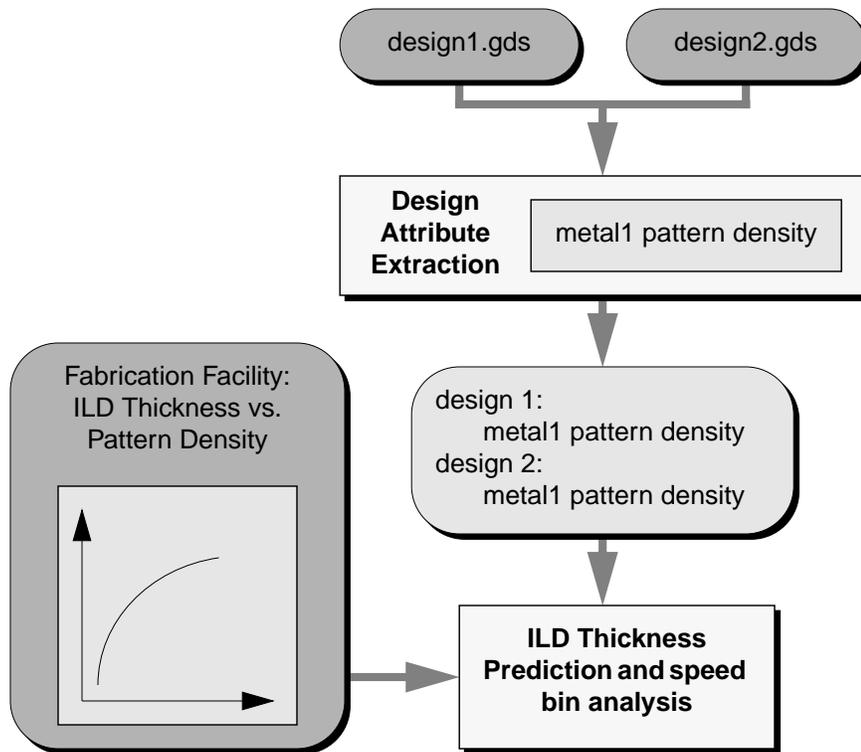
Figure 8. Task and data flow for metal1 pattern density extraction.
