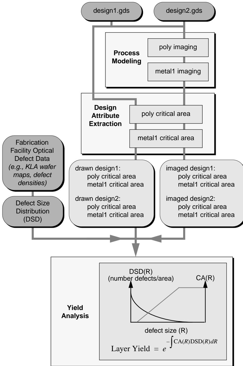
Figure 4. Task and data flow for critical area extraction for two designs, with and without process modeling. The end result of the flow is a set of layer yield predictions for the drawn and imaged models of the poly and metal layers of each design. (User input data is highlighted with darker shading.)
