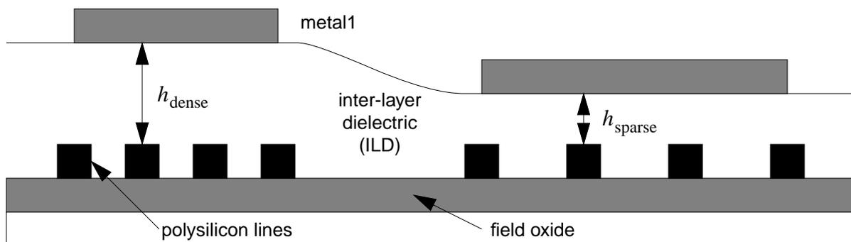
**Figure 7.** The effect of material pattern density on overlying dielectric thickness planarized by chemical mechanical polishing.
