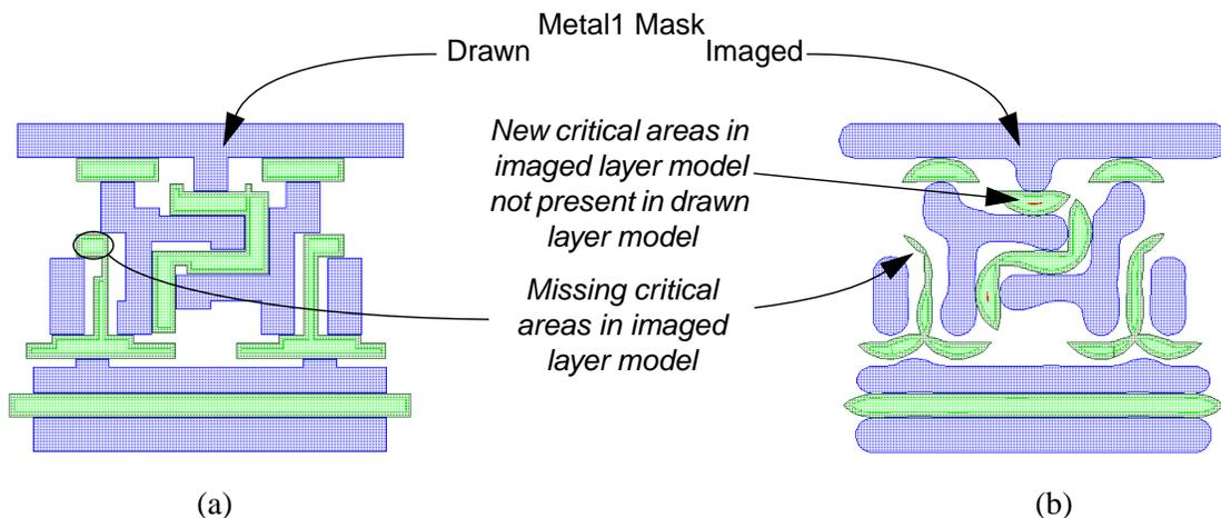
**Figure 5. The effect of aerial imaging simulation on critical area predictions. The concentric contours shown in each plot represent critical areas for decreasing defect sizes. Not only do certain critical areas disappear when using imaged layers, other critical areas are created for smaller defect sizes due to bloating of wire end-stubs.**
