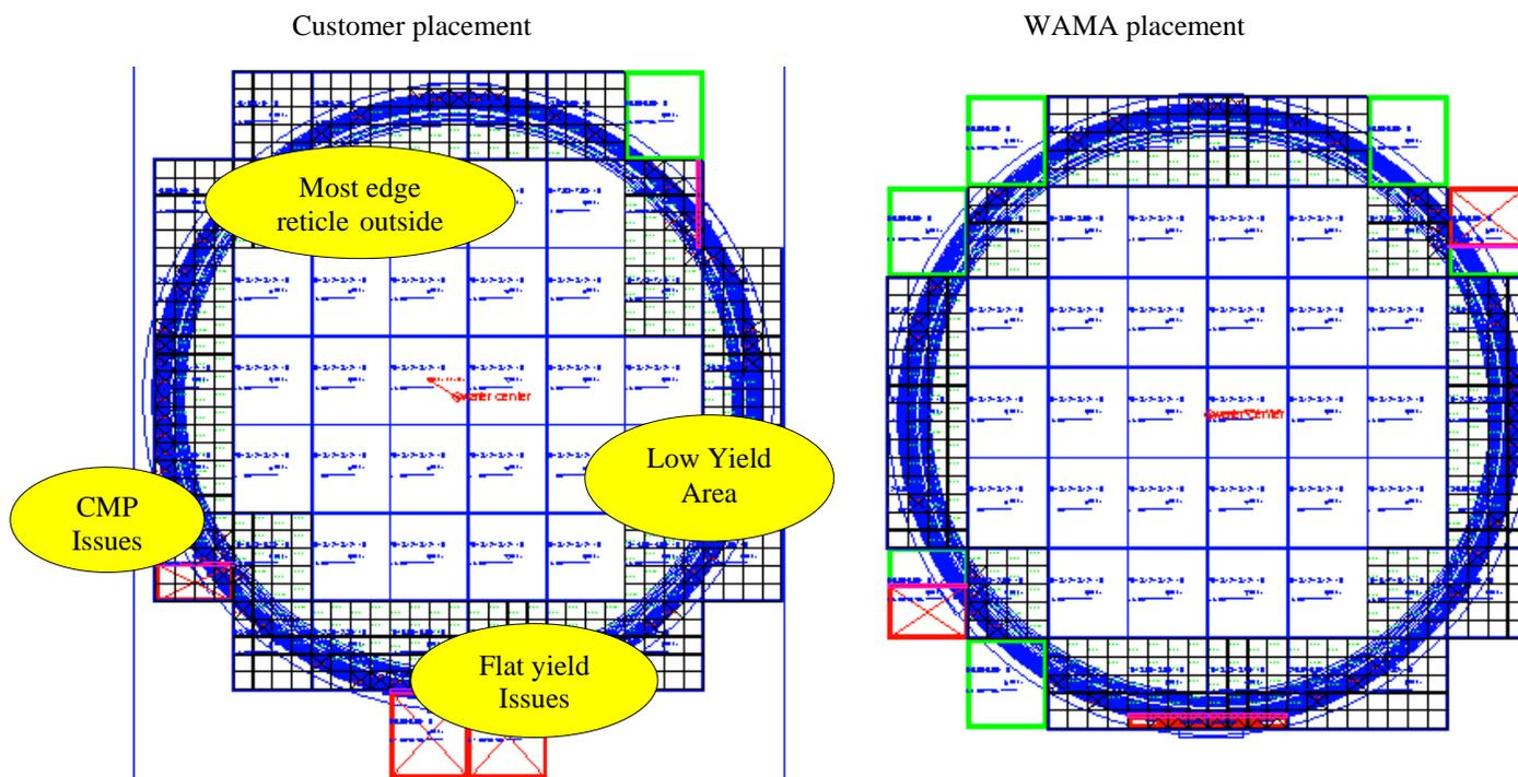
**Figure 4: Side-by-side placement before and after WAMA optimization. This example shows an improvement of more than 5% in the number of die-per-minute that the fab can generate for this product.**
