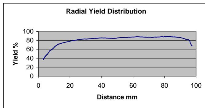
**Figure 3: This graph represents the average radial yield from the edge of the wafer.**
