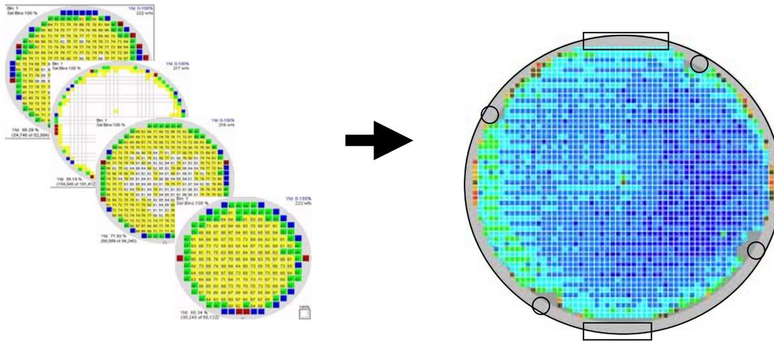
**Figure 2: Wafer process map, stacked map of multiple products of the same process.**
