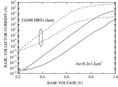
Fig. 7. Typical Gummel plot for one and 24,000 HBTs at  $V_{CB}=0$ .
