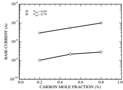
Fig. 4. Measured Base Current at two different Base-Emitter voltages as a function of Carbon Mole Fraction.  $V_{CB} = 0V$
