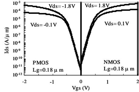
Fig. 9. Drain current ( $I_{ds}$ ) vs. gate voltage ( $V_{gs}$ ) characteristics of 1.8-V NMOS and PMOS
