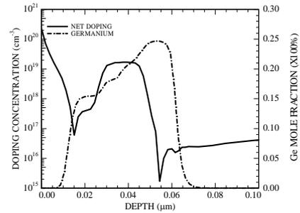
Fig. 3. SIMS profiles for net doping and germanium concentration for a typical HBT
