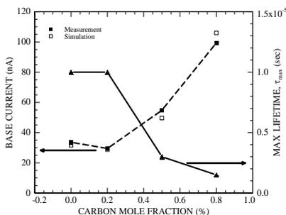
Fig. 10. Simulation results of base current (@  $V_{BE} = 0.7\text{V}$ ) as a function of carbon dose after tuning of  $\tau_{\text{max}}$
