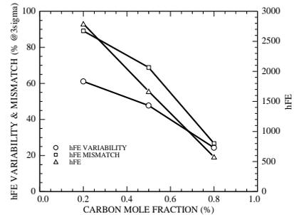
Fig. 5. Measured hFE, together with its variability and mismatch as a function of carbon concentration in the base layer
