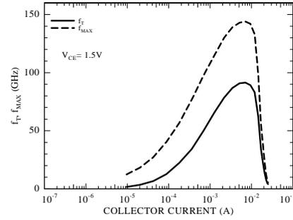
Fig. 8. Cut off frequency and maximum oscillation frequency vs. collector current.
