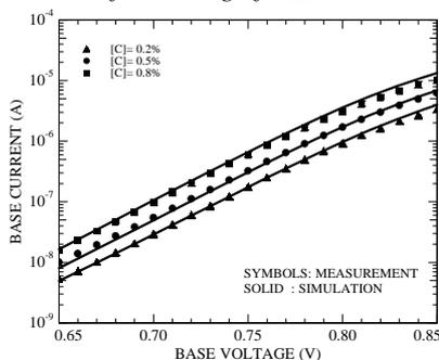
Fig. 11. Simulation of Gummel plots for base current at different carbon
