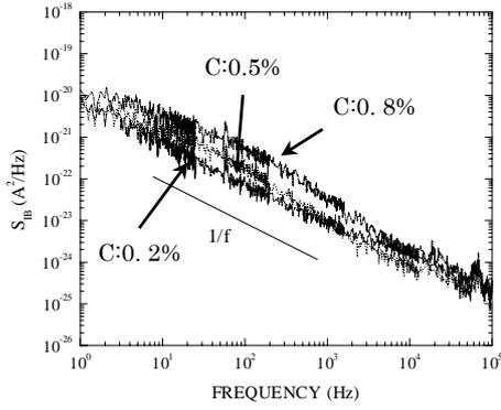
Fig. 6. Power spectral density of base current noise versus frequency for HBTs on different carbon content.
