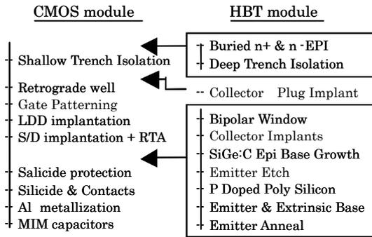
Fig. 2. Simplified fabrication process
