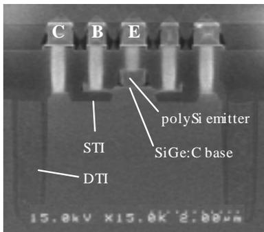
Fig. 1. SEM cross section of the HBT
